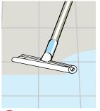
On an untreated, clean, dry floor apply a thin coat with seal applicator/clean soft brush.
