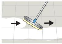
Pensure floor is free from debris/dust before applying a second coat. Apply in opposite direction to the first. Leave a 2.5-5cm gap from the edge.
